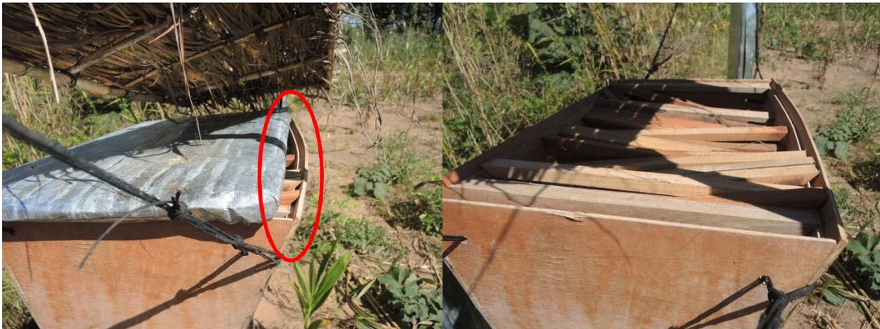
Fig. 16 and 17- Expansion of 6mm plywood after 2 months
