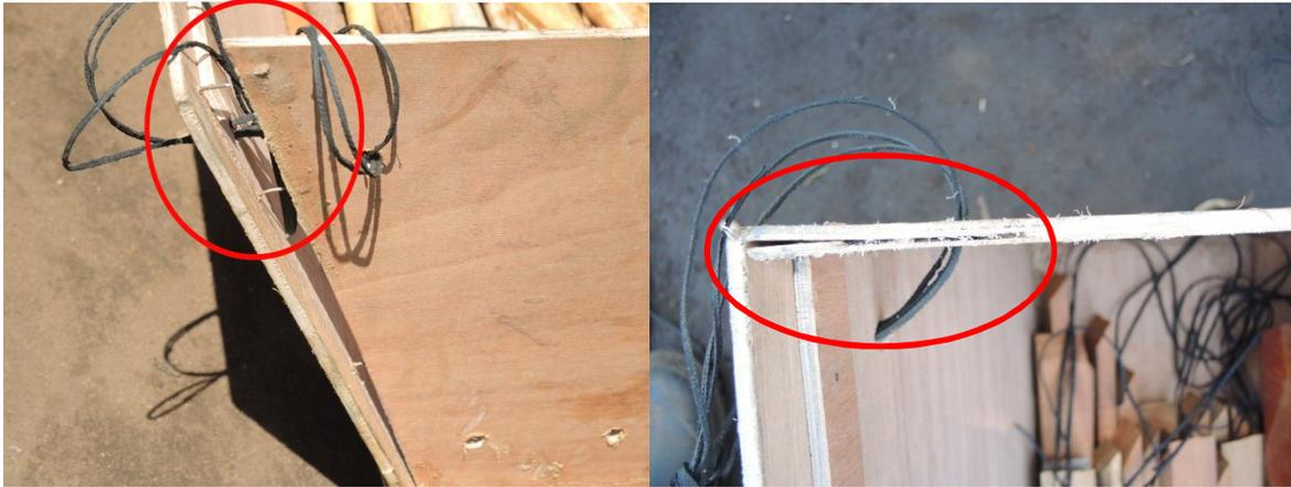
Fig. 14 and 15- Nails problems with 6mm plywood
