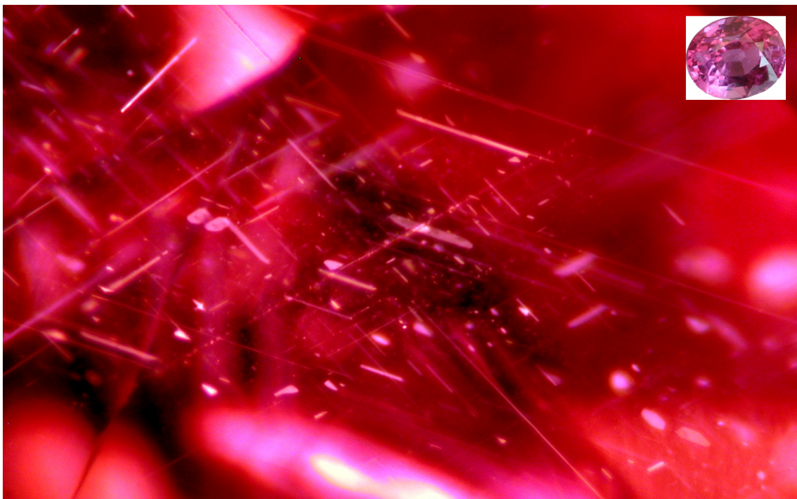
Figure 10: Silk in unheated 2.326cts Niassa ruby: It is clearly composed of elongated or short broad hexagonal like platelets and of long or short needles (Dark field illumination, 50x) Photo: V. Pardieu
