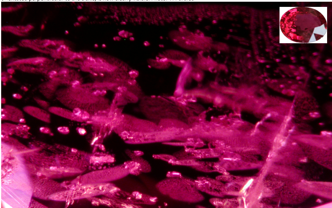
Figure 14, 2009: Plane of negative crystals associated with secondary healed fissures in a 1.510cts Niassa unheated ruby. (Dark field illumination, 30x) Photo: V. Pardieu
