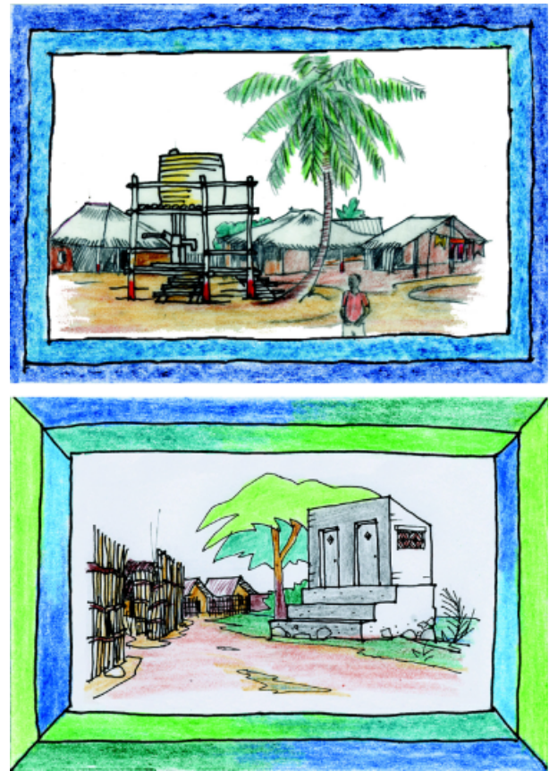
Figure 6 Cards illustrating examples of the flood proofing of rural water supply and sanitation infrastructure.
