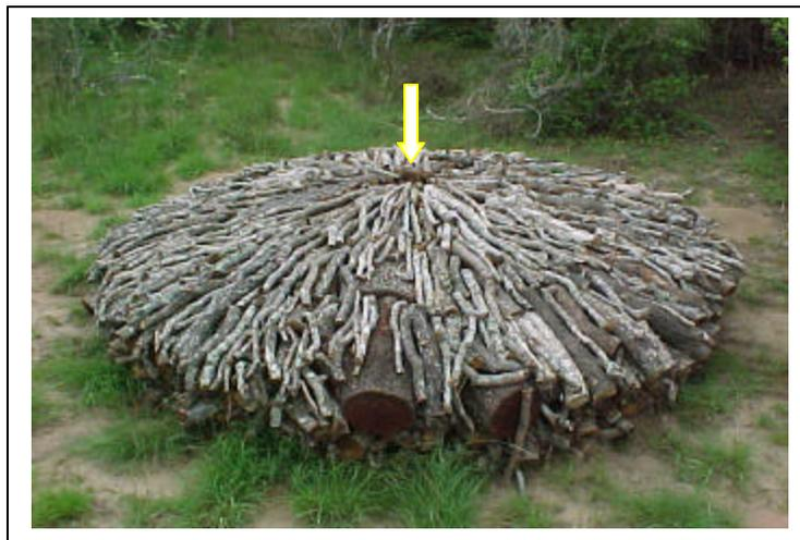
**FIGURA 12** LENHA ARRUMADA RADIALMENTE NO FORNO REDONDO COM A SETA A INDICAR O LOCAL ONDE SE VAI INTRODUIZIR O FOGO.
