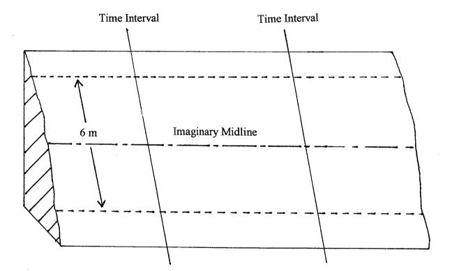
Figure 3. The "Horizontal Transect" survey technique employed by the programme for subtidal surveys
