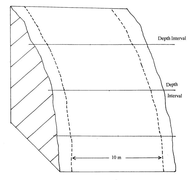
Figure 4. The "Vertical Transect" survey technique employed by the programme for subtidal surveys
