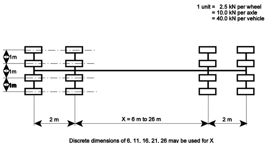
**Figure 2.2: Type NB loading**
