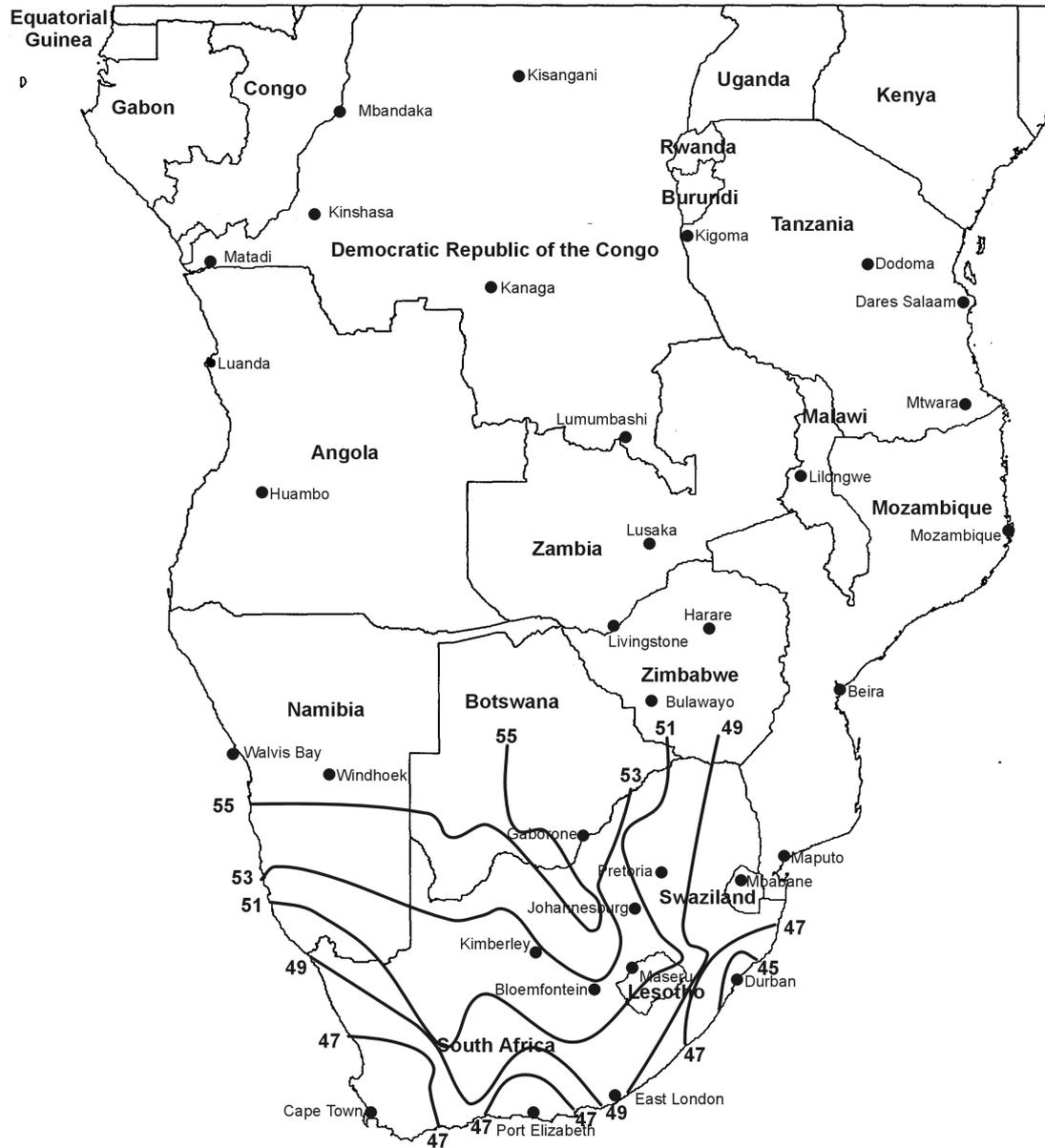
Figure 4.2: Isotherms of minimum shade temperature (in °C) for 50 year return period
