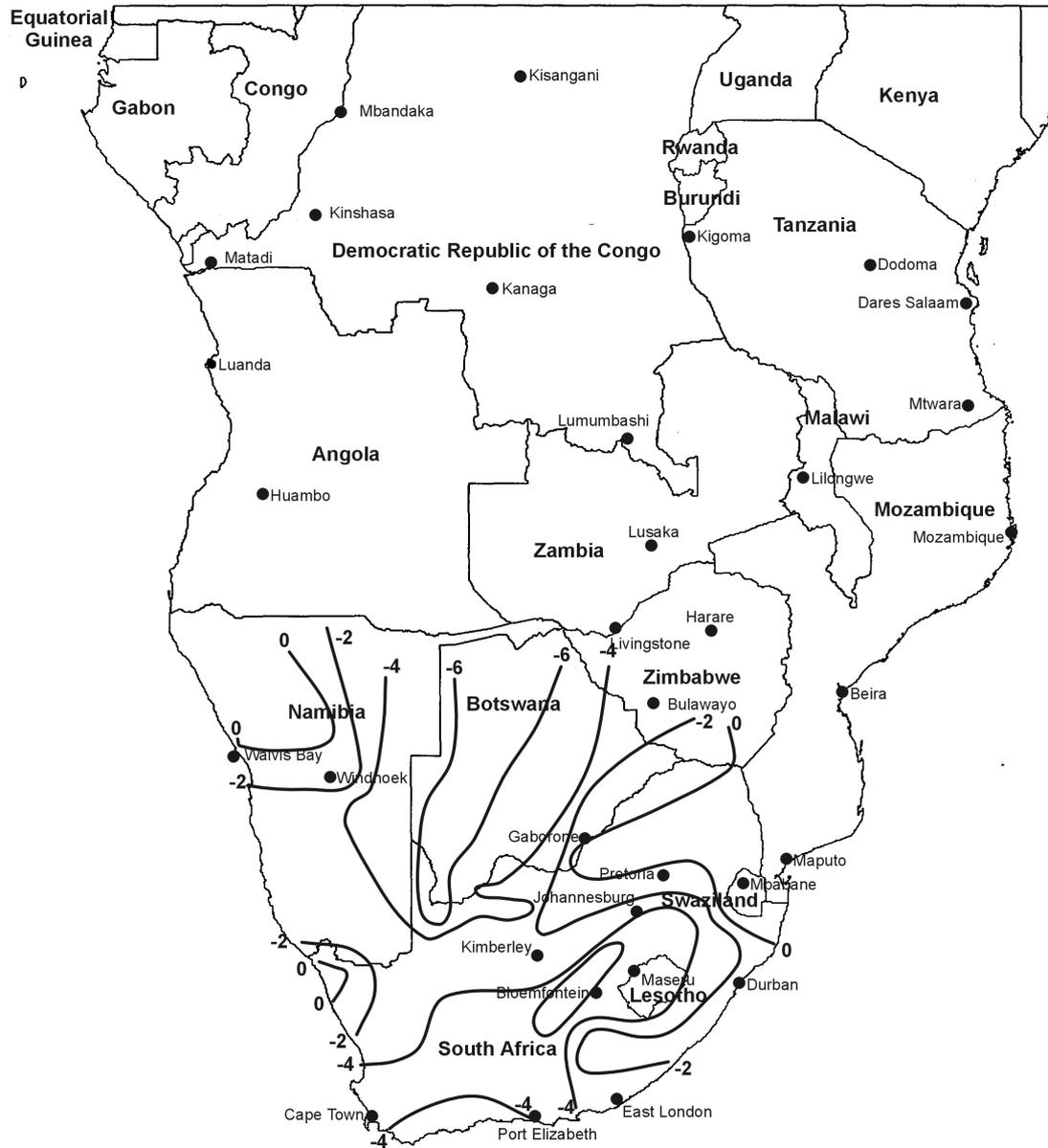
**Figure 4.1: Isotherms of minimum shade temperature (in °C) for 50 year return period**
