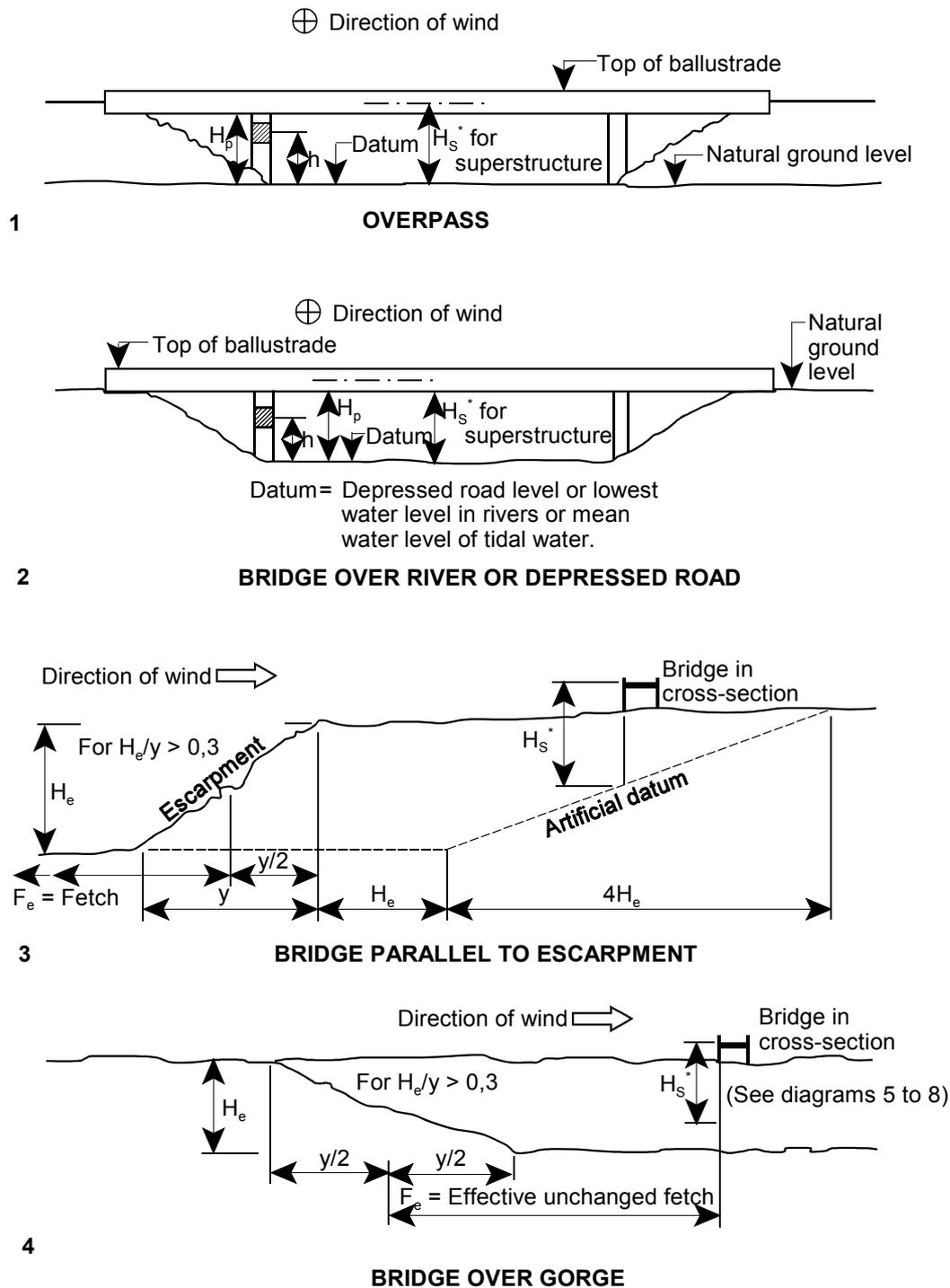
\* The values indicated are the effective heights for winds transverse to the structure assuming that the ground profile (fetch) is largely unchanged in the upwind directions for a distance  $F_e = H_s^2 / 10$ .
