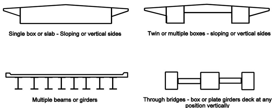
**Figure 3.9: Typical bridge cross-sections to which Figure 3.8 applies**
