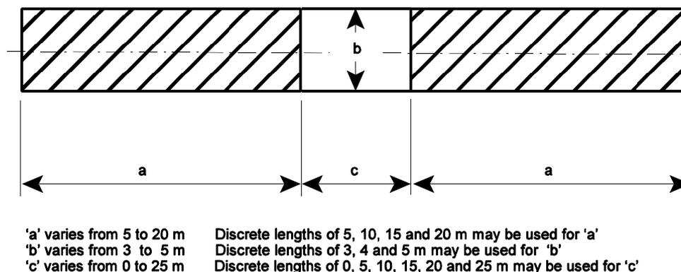
**Figure 2.3: Type NC-36 X 5 X 40 loading**
