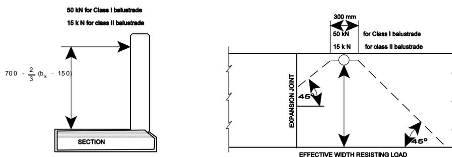
Figure 3.4: Forces on concrete parapet walls
