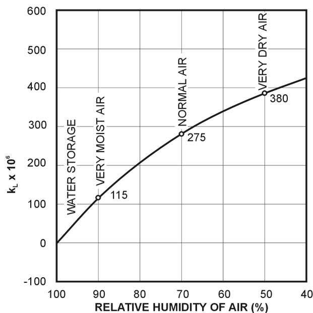
Figure E.6: Coefficient  $k_L$  (environmental conditions for shrinkage)
