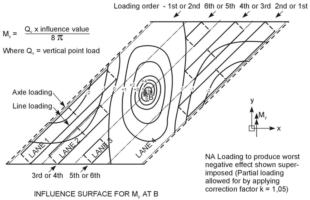
**Figure A.3: NA line and axle loading on skew bridge**
