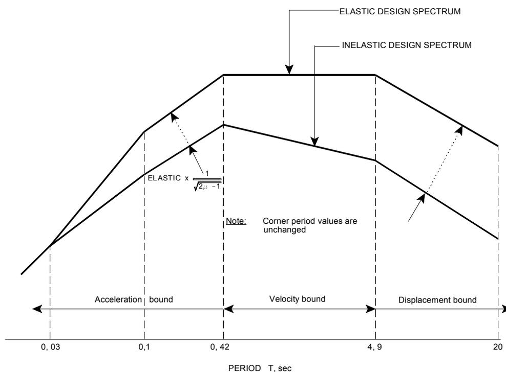
**Figure 3.14: Transformation from elastic to elastic - plastic design spectrum**
