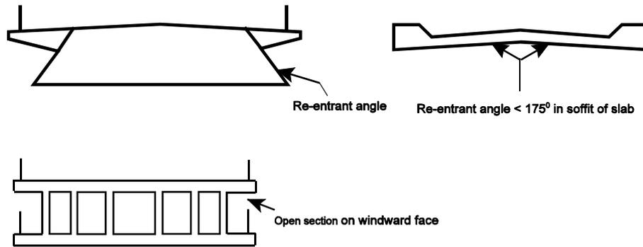
**Figure 3.10: Typical bridge cross-sections that require wind tunnel tests**
