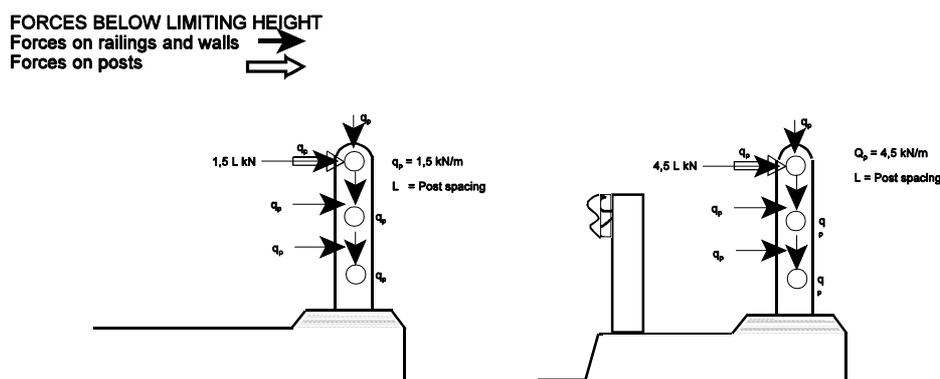
**Figure 3.3: Forces on Class II balustrades**
