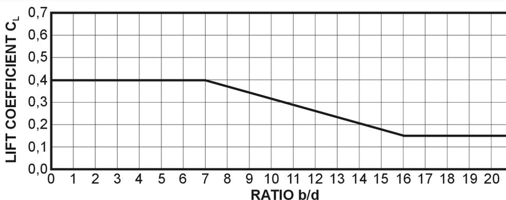
**Figure 3.11: Lift coefficient CL**
