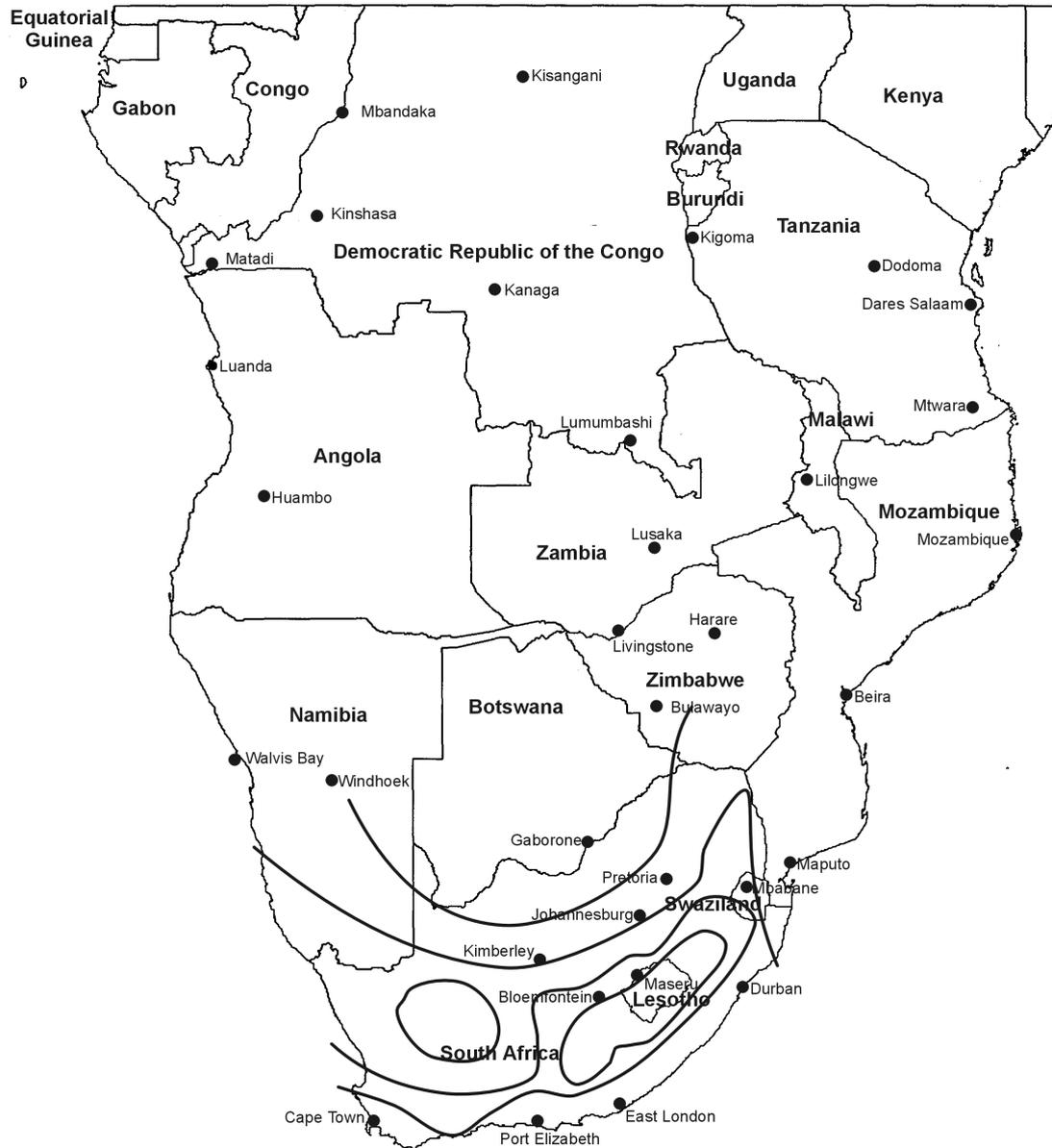
**Figure 3.5: Isotachs of estimated mean hourly wind speeds in m/s appropriate to a height above ground level of 10 m in open level country and a 100-year return period**
