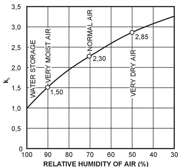
Figure E.1: Coefficient  $k_L$  (environmental conditions) for creep
