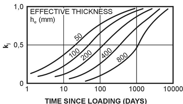
Figure E.5: Coefficient  $k_j$  (variation as a function of time)
