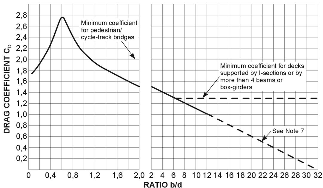
Figure 3.8: Drag coefficient  $C_D$  for superstructures with solid elevation
