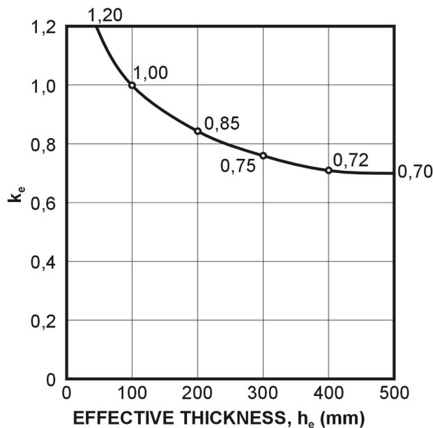
Figure E.4: Coefficient  $k_e$  (effective thickness) for creep
