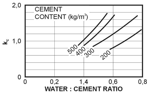
Figure E.3: Coefficient  $k_c$  (composition of the concrete)
