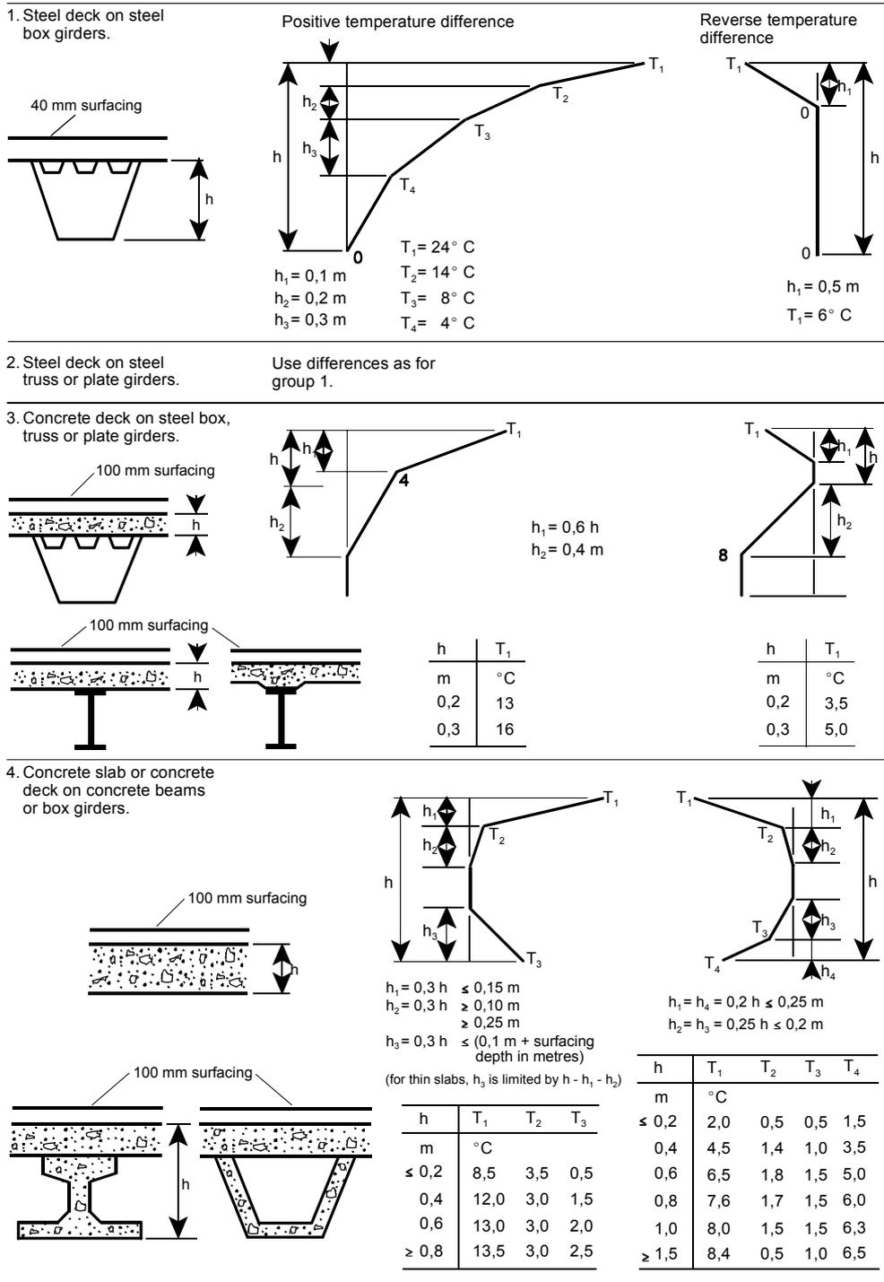
Figure 4.3: Temperature difference for different types of construction
