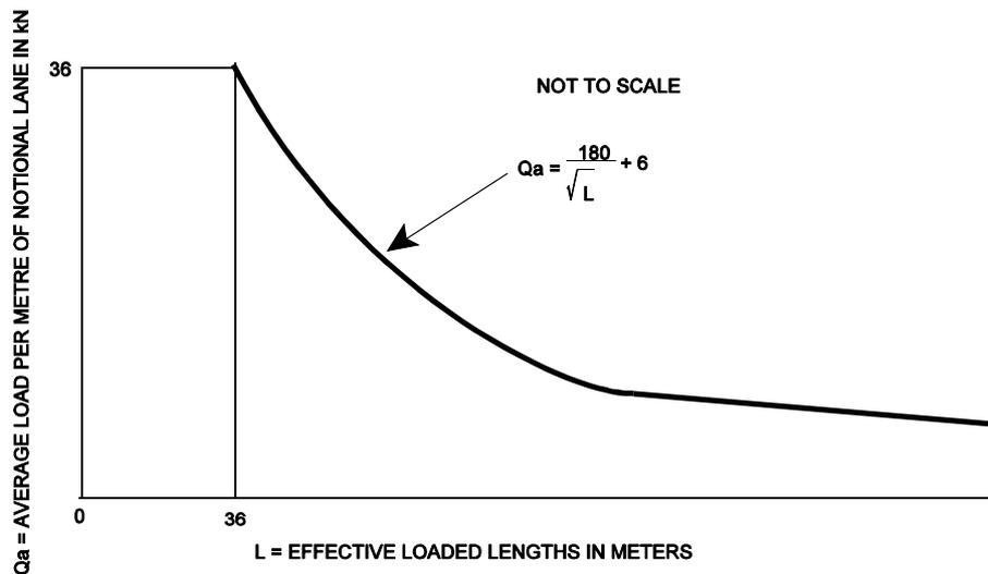
**Figure 2.1: Loading curve for type NA loading**
