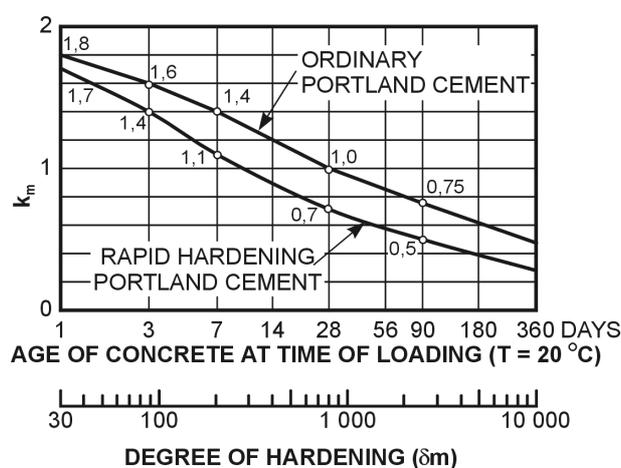
Figure E.2: Coefficient  $k_m$  hardening (maturity) at the time of loading
