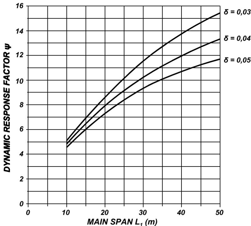
**NOTE 1.** Main span  $L_1$  is shown in Table 18
