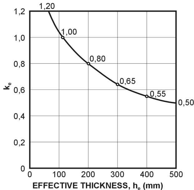
**Figure E.7: Coefficient  $k_e$  (effective thickness) for shrinkage**
