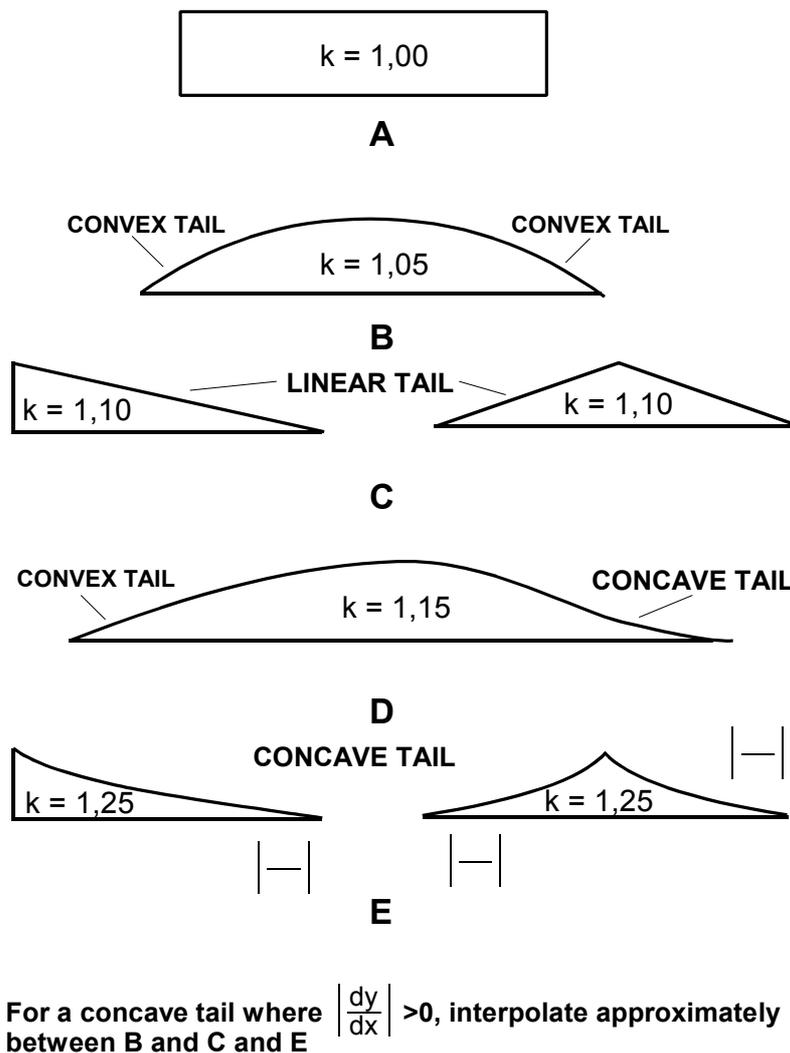
**Figure A.1: Correction factors for typical shapes of influence lines**
