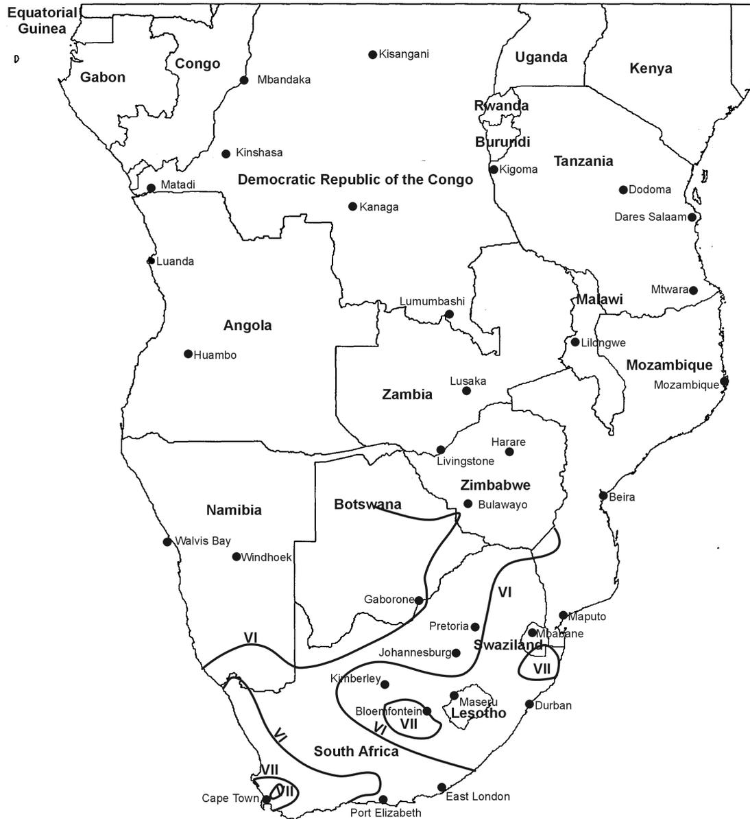
**Figure 3.12: Earthquake intensity zones in terms of modified Mercalli scale**
