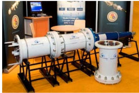
Figure 4.10: HRC Hydro Renewables Connector designed by Hydro Group ([21])
