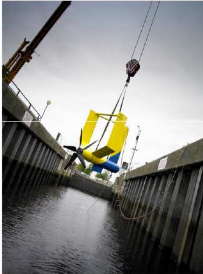
Figure 53 Testing of the Evopod at the Tees barrage [68]
