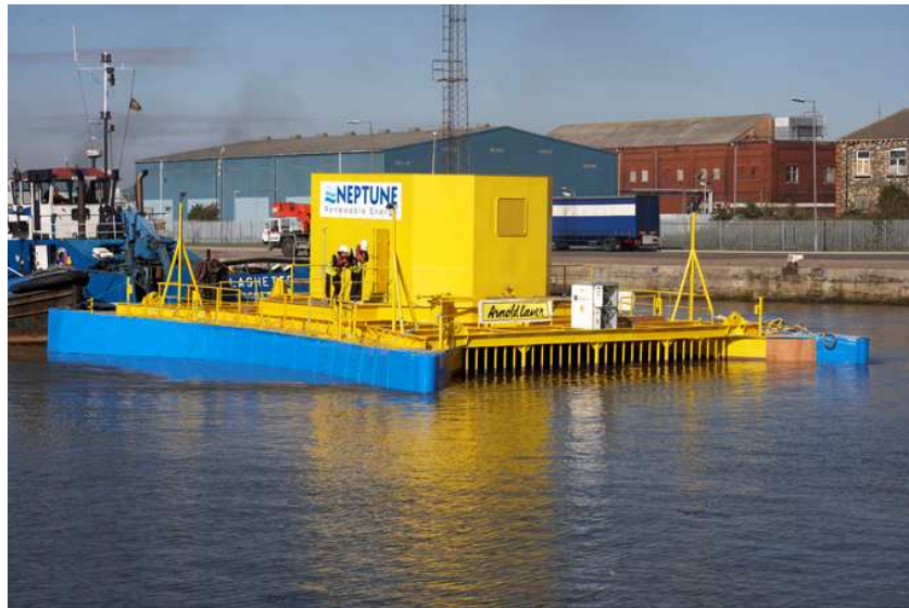
Figure 61 NREL Proteus device in the Humber [84]
