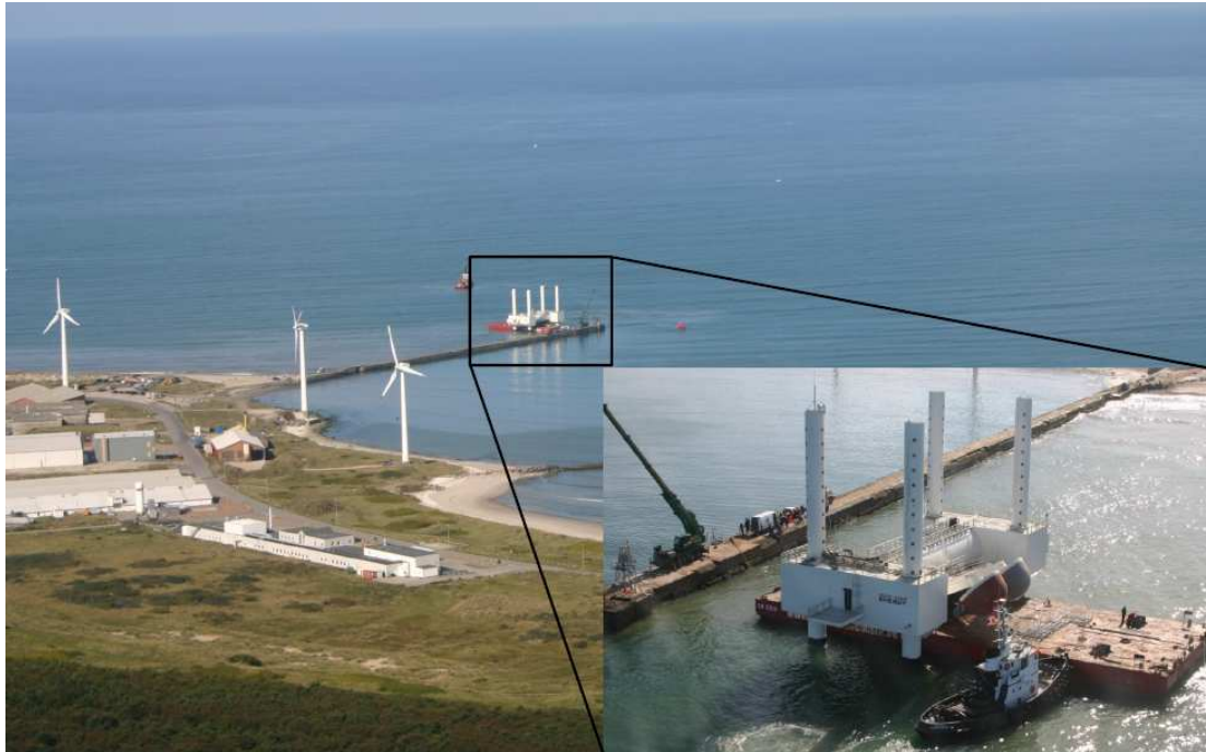
Figure 14 1:2 Scale WaveStar device on test at Hanstholm[22]
