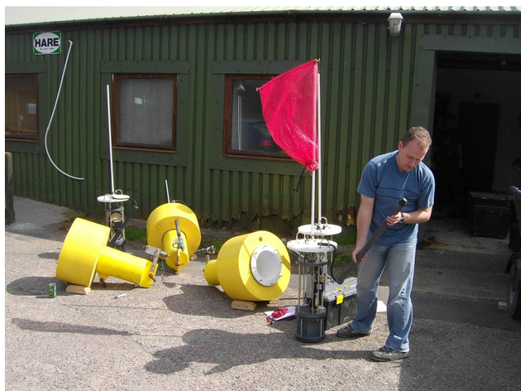
Figure 13: In air testing of VRAP-buoy system.
