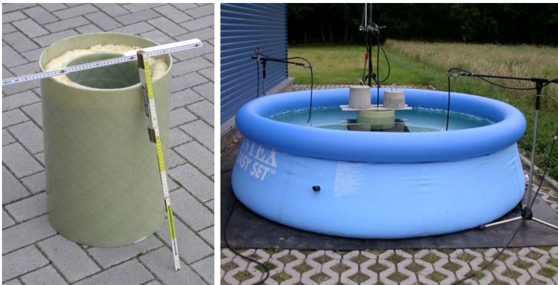
Figure 3-28. Double-wall model of a pile sleeve with a 50 mm foam layer and test setup with two hydrophones and a piezo-electric transducer as sound source inside the tube.
