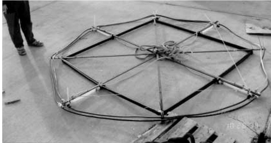
Fig. 3-16. Test setup by Vagle (2003). The outer ring has a diameter of 3 m and is supplied air by the square manifold in the centre.
