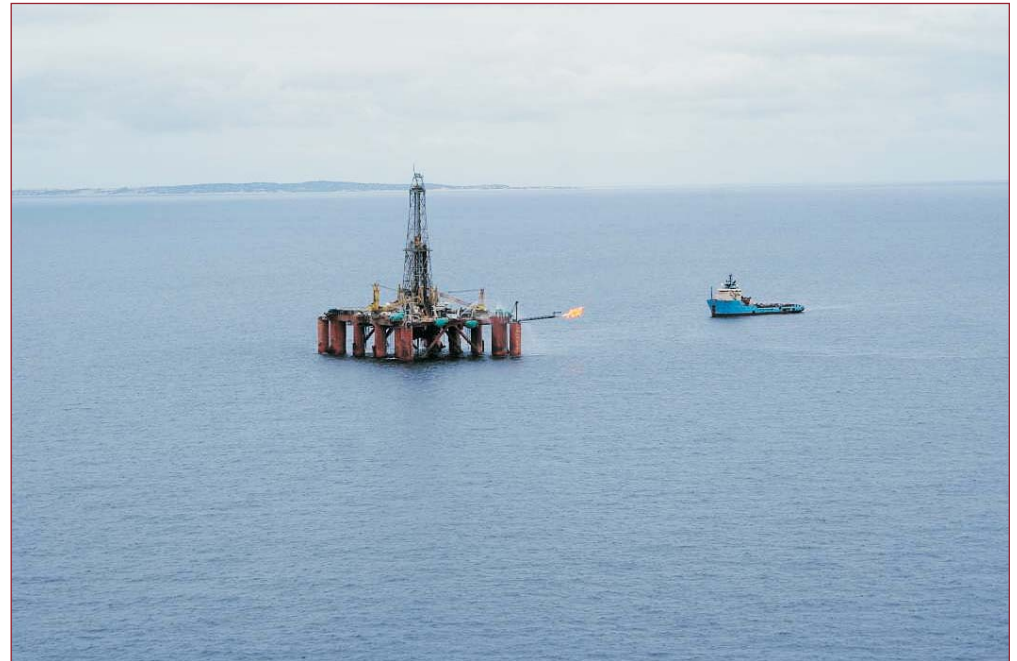
Figure 2: Semi-submersible Drilling Unit and standby boat during deep water exploration drilling, with Bazaruto Island in the background
