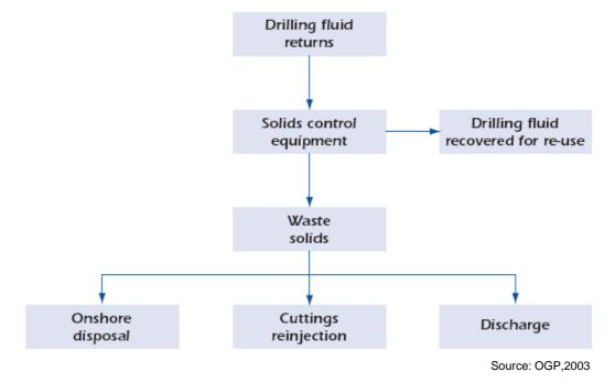
**Figure 16** Schematic Flow Chart Showing Separation of Cuttings from Drilling Fluids and Options for Drill Cuttings Disposal
