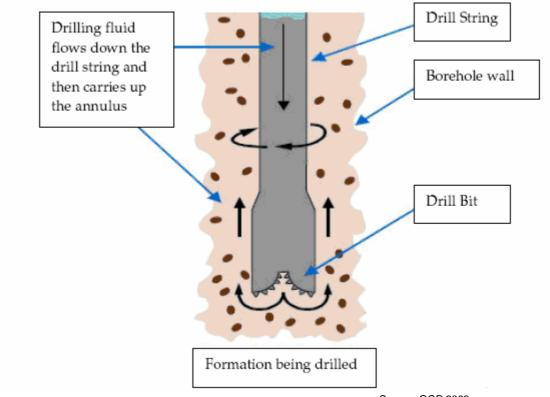
Figure 8 Circulation of fluids in the drill bit
