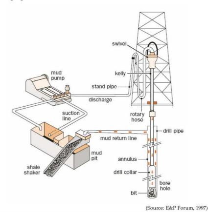
Figure 7 Main features of a drilling rig
