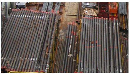
Figure 15 Pipes used for casing
