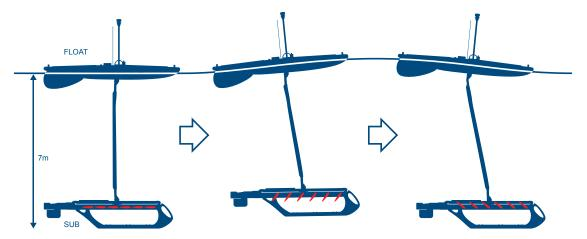
A rising wave lifts the Float, causing the tethered Sub to rise. The articulated wings on the Sub are pressed down and the upward motion of the Sub becomes an up-and-forward motion, in turn pulling the Float forward and off the wave. This causes the Sub to drop, the wings pivot up, and the Sub moves down-and-forward. This process is repeated again and again as long as there is wave motion on the surface, even the smallest amount.
