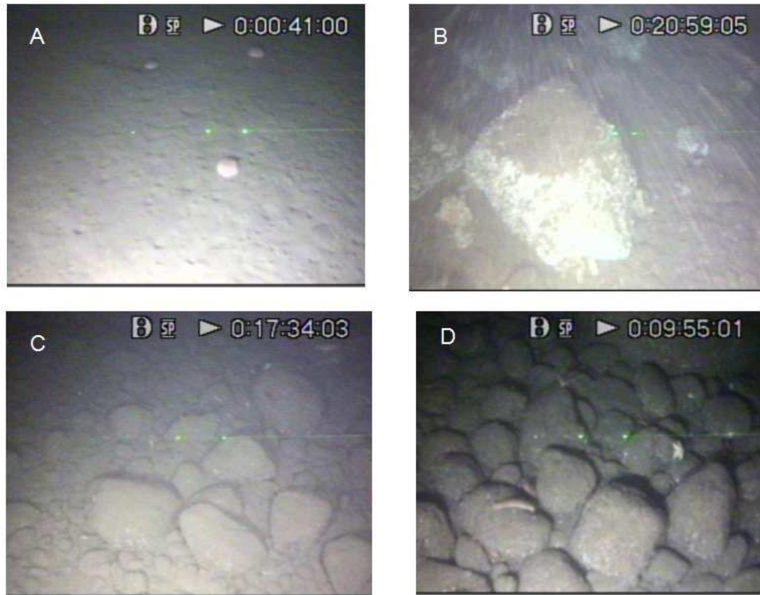
Figure 3. Frame grab images of bottom types. Frame grabs show examples of bottom types observed in the survey: A) hummocky sand-mud (SM) substrates; B) scattered boulder on pebble cobble (PB1); C) cobble with scattered boulder (CB1); and D) stacked boulder (BB3). Laser points projected onto the bottom by the 3-beam QMS were used to estimate the size of objects. Rightmost and leftmost laser points were two feet apart.
