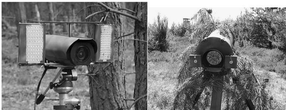
Fig. 2 Automatic IR video camera with IR diode panels ( left ) and high-power IR-emitting diodes
